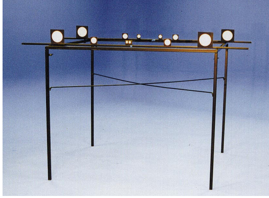
Figure 12. Lens calibration targets: nodal point and field of view.
